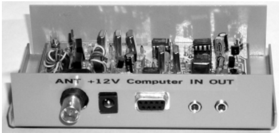
A prototype Warbler mounted in an LMB-139 enclosure ... perfect fit!
