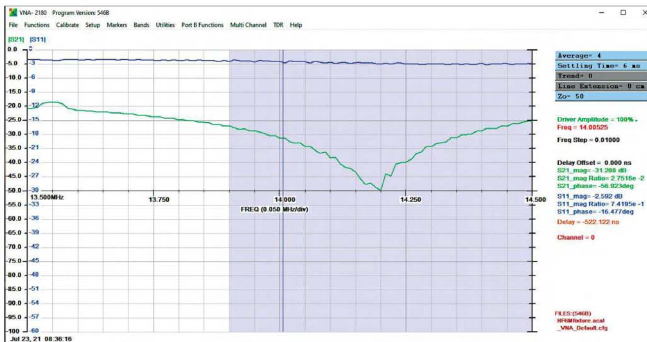
Figure 5 — The trap isolation measurement.
